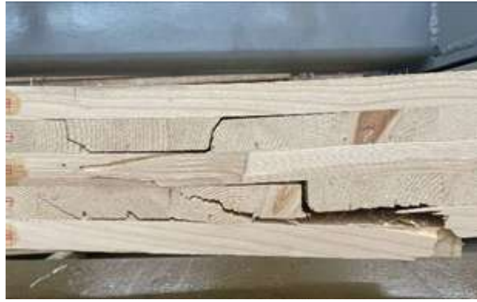
Figure 9.48: Typical failure mode of Series A panels (specimen A1)
