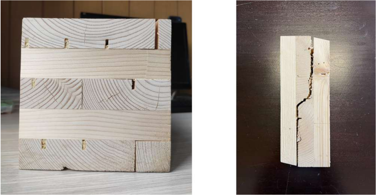
Figure 1.1: Cross laminated timber (CLT) panel (left) and typical rolling shear failure mode of CLT panel (right)
